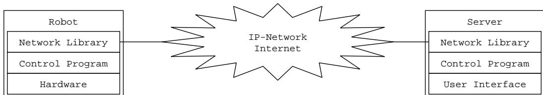
This communication has to be bidirectional because it has to be possible to get data from the robot. This is important to get the acknowledgement for a command, get knowledge of the environment of the robot and to monitor the
